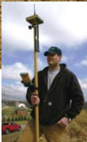
Jim McGowan of McGowan-Stauffer Inc. checks grades with Topcon's HiPer+ survey system to analyze the site for design adjustments.
